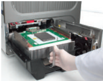
▲ LightCycler® 480 Thermoblock for 96 or 384 wells, easily exchanged by users within minutes.
